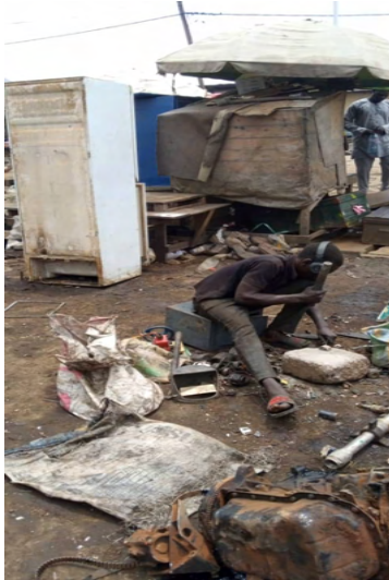
Dismantling: Breaking the electronic waste into pieces to extract valuable material for retail or reuse. E.g., Copper, gold, Aluminum
